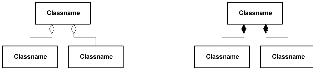
Figure 4g: Aggregations (left) and compositions (right) allow the clearly arranged depiction of complex systems
