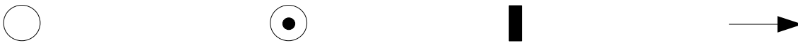
Figure 2: An unmarked local state, a marked local state, a local transition and a relation between a state and a transition (from left to right)
