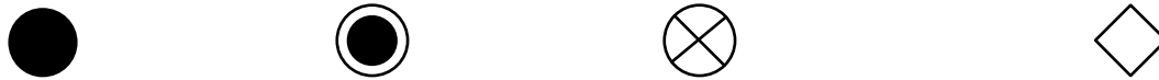
Figure 7d: The control nodes: initial node, final activity node, final-follow node and decision/merge node (from left)
