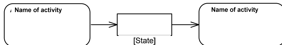
Figure 7c: The object flow considers the states that are reached through executing the activities
